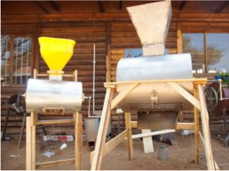
First prototype of the bean thresher (left) and second prototype (right) incorporating community's feedback, which indicated a need for a machine with larger capacity, and hooks to hold the sack at the outlet.
