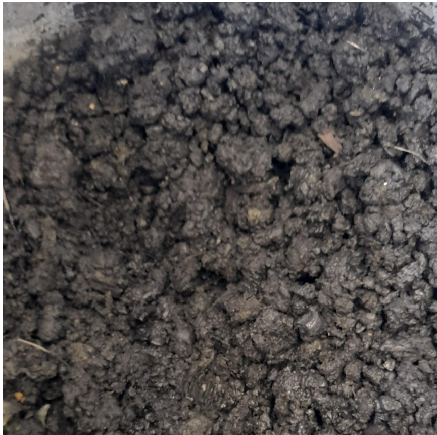
Picture showing activated biochar made from charcoal and sheep poo slurry.
