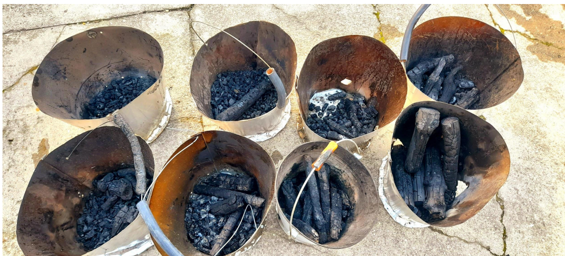
Pictures showing participants using their small metal bucket kilns to carbonize slash at the Uawa Beach and the biochar they produced.
